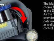
The MultiSense SL is the sensor of choice for the Atlas humanoid robots in the DARPA Robotics Challenge (DRC). As the "head" of the humanoid, the SL provides the majority of perceptual data used for teleoperation as well as automated control.
